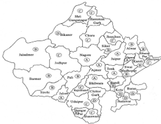
Fig. 3: Categorization of fluoride affected districts of Rajasthan Category A: 50% and above villages have excess of fluoride (very serious). Category B: 25-50 % villages having excess fluoride (serious). Category C: 10-25 % villages having excess fluoride (less serious). Category D: Below 10% villages having excess fluoride (insignificant).
